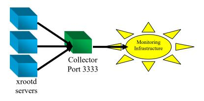
of xrootd servers send their statistics to a collector machine listening at port 3333. The collector merges all of the data streams and sends a selection of the desired data to the monitoring infrastructure.
