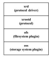
The particular components that need to be configured are the file system plug-in (**ofs**) and the storage system plug-in (**oss**). The relationship between **xrootd** and the plug-ins is shown on the left. The protocol driver (**xrd**) runs the **xroot** protocol which, in turn, utilizes the file system plug-in that, itself, relies on the storage system plug-in. Collectively, this is called **xrootd**, the executable that encapsulates all of the components.
