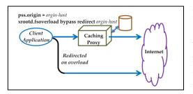
Finally, you can also use a forwarding mode or combination mode caching proxy without using a firewall. However, the xrootd layer must be told that client can be redirected to their original destination should a forwarding location be specified. This is done by adding
