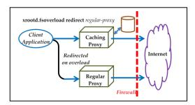
The graphic on the left shows a typical proxy that sits behind a firewall. All access to the internet requires that a proxy server be used. Normally, clients connect to the caching proxy server. This can be a direct mode, forwarding mode, or combination mode proxy. It doesn't really matter. When the caching layer indicates
