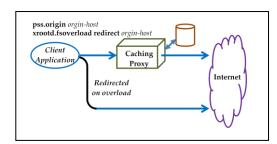
If your site does not have a firewall but you still want to cache data closer to your site; you would also setup a caching proxy server. The **pss.origin** would specify the host that normally clients would connect on the internet. If the caching proxy becomes overloaded the **xrootd.fsoverload** directive
