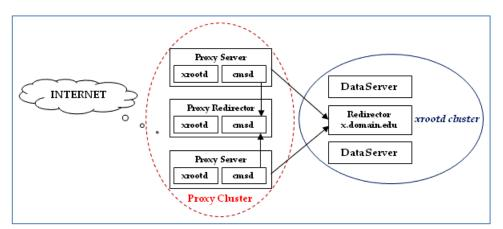
configure a proxy redirector. The initial point of contact for external clients is the proxy redirector. This is shown in the adjacent diagram.
