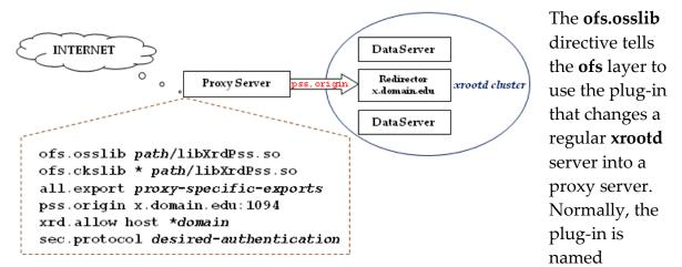
"libXrdPss.so". You must specify the location of this shared library plug-in. To support checksum calculations you must also indicate that the checksum manager is a proxy as well. This is done loading the proxy library via the **ofs.ckslib** directive.
