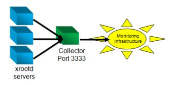
This picture illustrates the general scheme most installations use to gather summary statistics and insert them into their monitoring framework. Here a number of xrootd servers send their statistics to a collector machine listening at port 3333. The collector merges all
