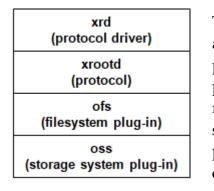
The particular components that need to be configured are the file system plug-in (**ofs**) and the storage system plug-in (**oss**). The relationship between **xrootd** and the plug-ins is shown on the left. The protocol driver (**xrd**) runs the **xroot** protocol which, in turn, utilizes the file system plug-in that, itself, relies on the storage system plug-in. Collectively, this is called **xrootd**, the executable that encapsulates all of the components.
