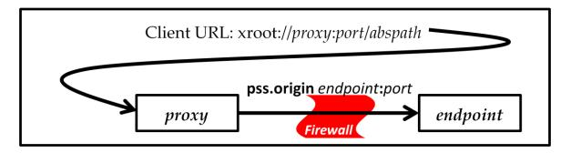
In the diagram the client present a URL that identifies the proxy server or proxy cluster. The proxy then contacts the data origin, a particular endpoint, on behalf of the client and performs the requested operation. The endpoint can be an actual server or a cluster redirector. This mode is suitable for incoming connections to a fire walled cluster or outgoing connections to a particular data source.
