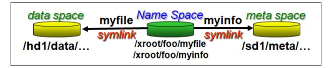
In this example, spaces have been used to establish high performance space (i.e. ssd) and low performance space (i.e. hard drive) and provide the ability for the client to choose which space to use without sacrificing a single uniform name space. Spaces can be used for any number of reasons like piecing together multiple file systems to provide a large pool of storage space that can grow as needed.
